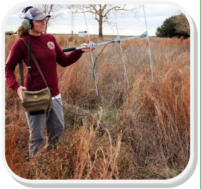
Above: Mandy Bellamy using a yagi antenna and receiver, to walk out to a radio collared chicken. Photo by Garet Litwiler
